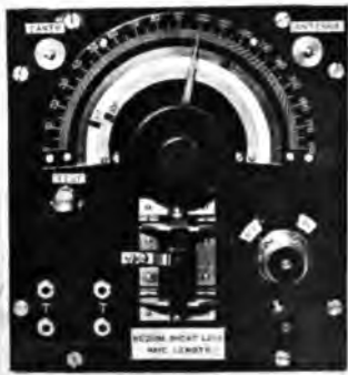
FIG. 47.—Box type receiver.
